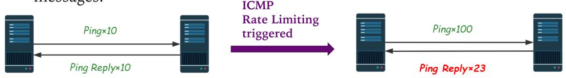
Usually, widespread ICMP rate limiting is considered to bring more challenges to IPv6 measurements (especially topology discovery), but the **global** ICMP rate limiting also opens up new side channels.
