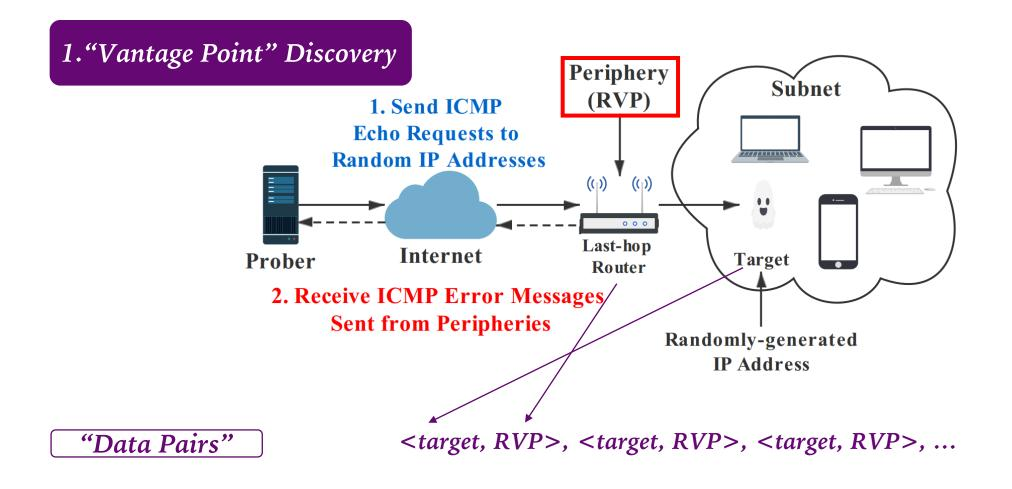
First, we perform active measurements to discover potential **remote "vantage points" (RVPs).** Though, they are not "vantage points" in the true sense. They are mostly others' routers.
